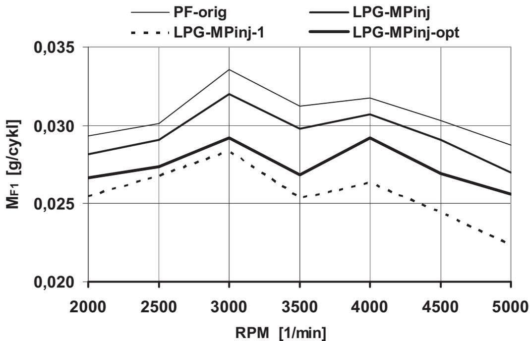
Fig. 10. The injected fuel quantities for full load conditions at running on PF and on LPG for different variants of the experimental engine they reflect the right functional coupling original ECU of PF engine on ECU Vialle fuel system for injection of the liquid LPG
