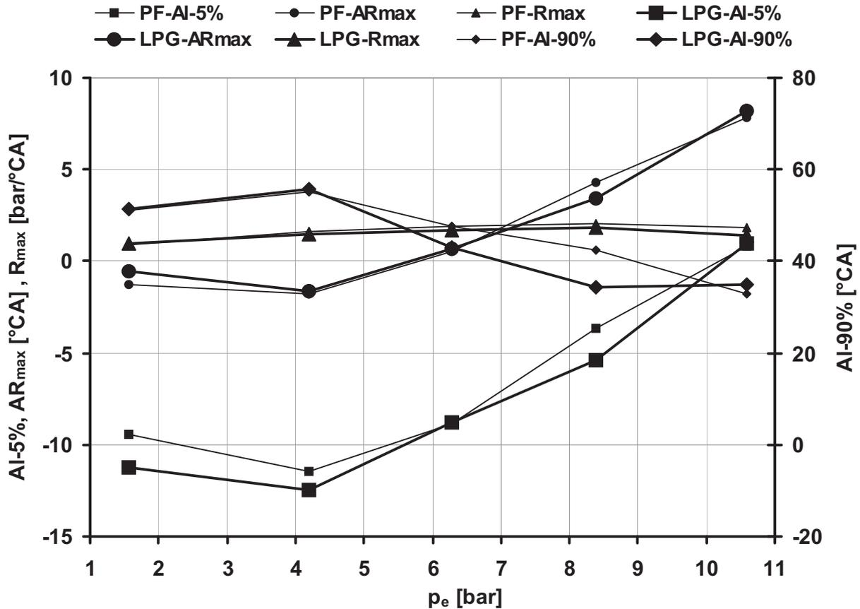
Fig. 9. The parameters of the course of mixture combustion at cylinder at running on PF and on LPG on load characteristic at RPM = 3000 1/min
