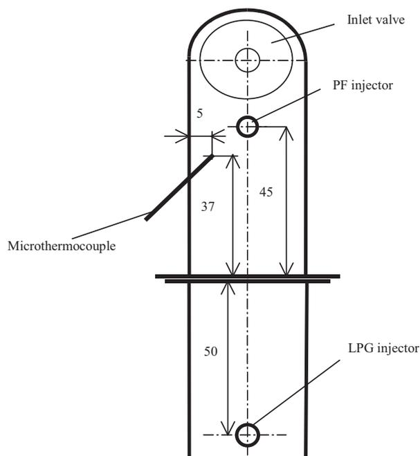
Fig. 2. The scheme of microthermocouple in the intake port in cylinder head for metering air (mixture) temperature before the intake valve. The scheme of dimension location for measuring temperature in the intake port of the engine (dimensions shown are reached at extended central axis of the port)
