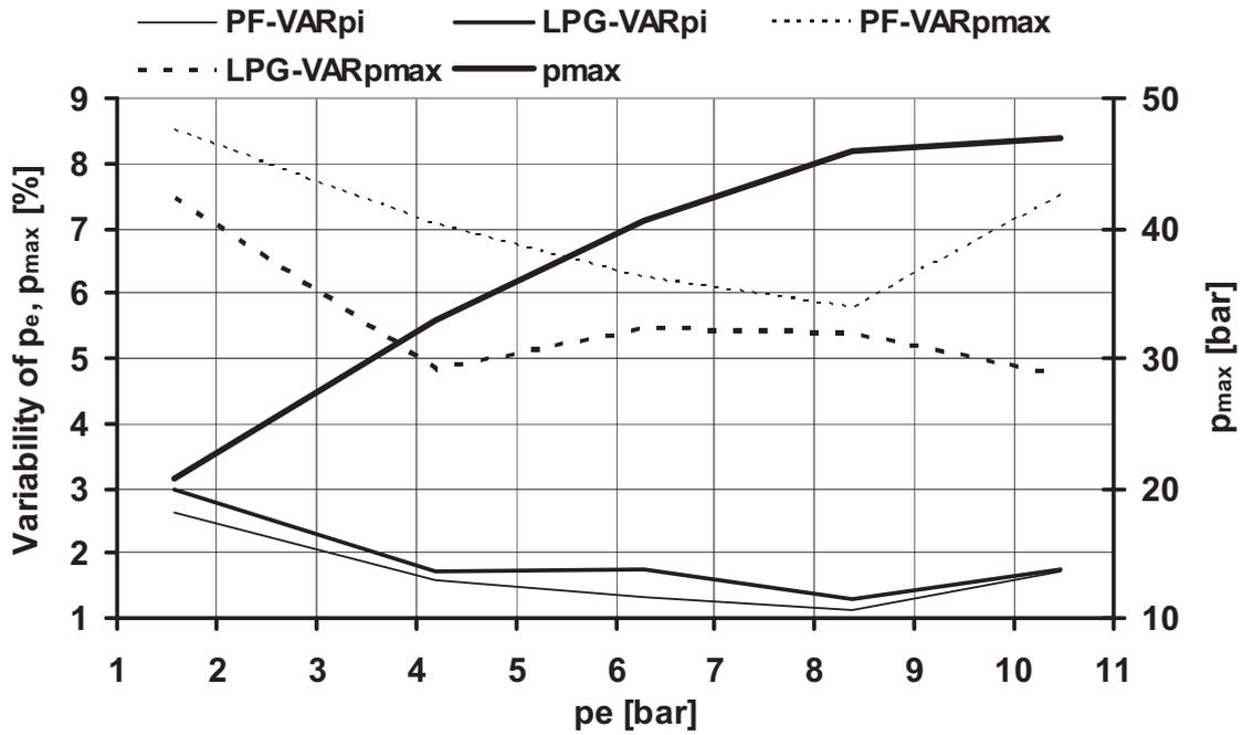
Fig. 8. Combustion peak pressures on load characteristic at RPM = 3000 1/min they have at engine running on PF and on LPG virtually like the same values, the parameters of the intercycles variability for PF and LPG they are for  $p_i$  as well comparable, the engine running on LPG has a somewhat lower values of intercycles variability for  $p_{max}$  (by using statistical processing of the set 150 sequential following cycles)
