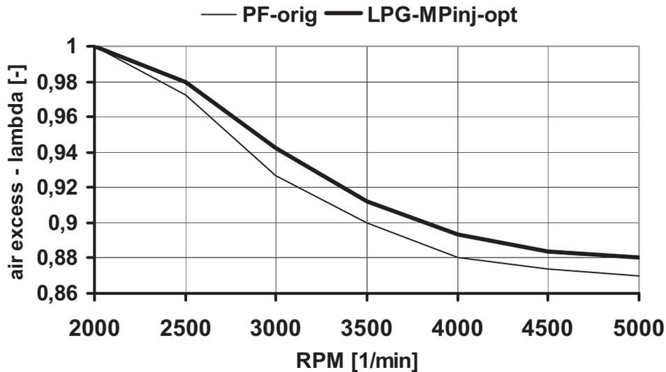
Fig. 6. The optimized governing of the mixture richness for full load conditions of the experimental SI engine with injection liquid of LPG to the intake manifold in face of intake port at cylinder head
