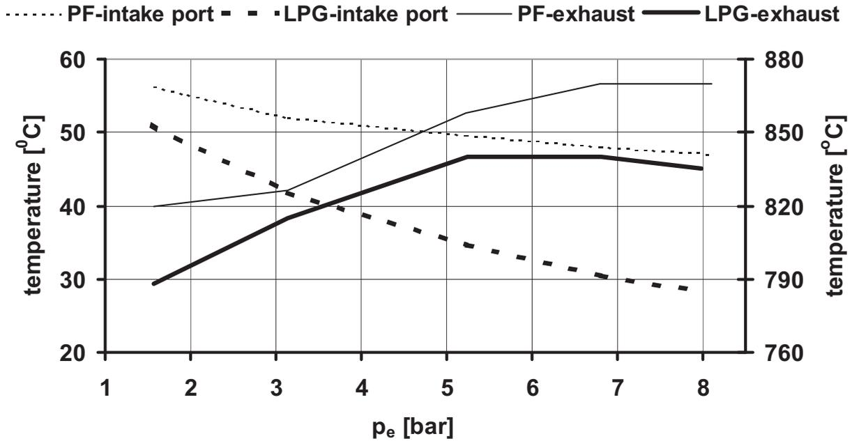
Fig. 4. Fresh mixture temperature in intake port at cylinder head and exhaust gas temperature at 5000 rpm (the temperature in the intake port is determined as arithmetic mean of 16-18 recorded temperatures for each measurement point, the exhaust gas temperature there is calculated as arithmetic mean from several points at the end of each measurement mode)
