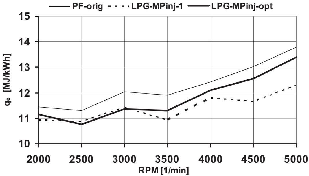
Fig. 11. Specific consumption of the heat on full load speed characteristic for different variants of experimental engine
